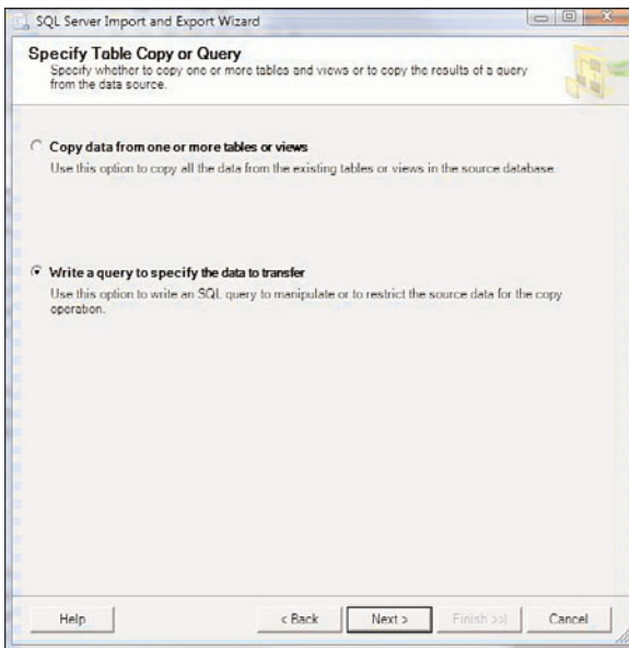
FIGURE 52.19 Specifying to use tables or a query for data transfer from the data source.
